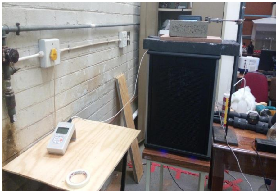
Figure. 5 Setup for Thermal Conductivity
