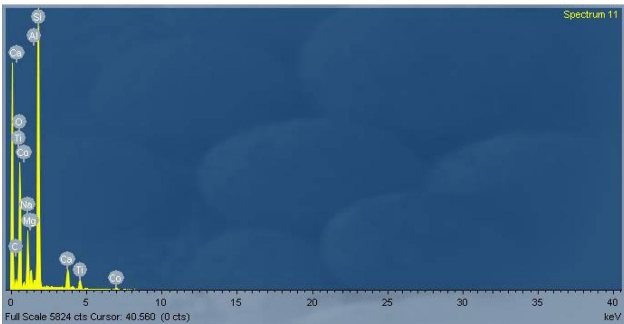
Figure 1c, EDS for TiO<sub>2</sub>/CoO core-shell thin film annealed at 573K
