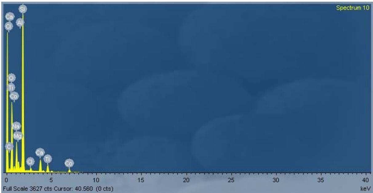
Figure 1b, EDS for TiO<sub>2</sub>/CoO core-shell thin film annealed at 373K
