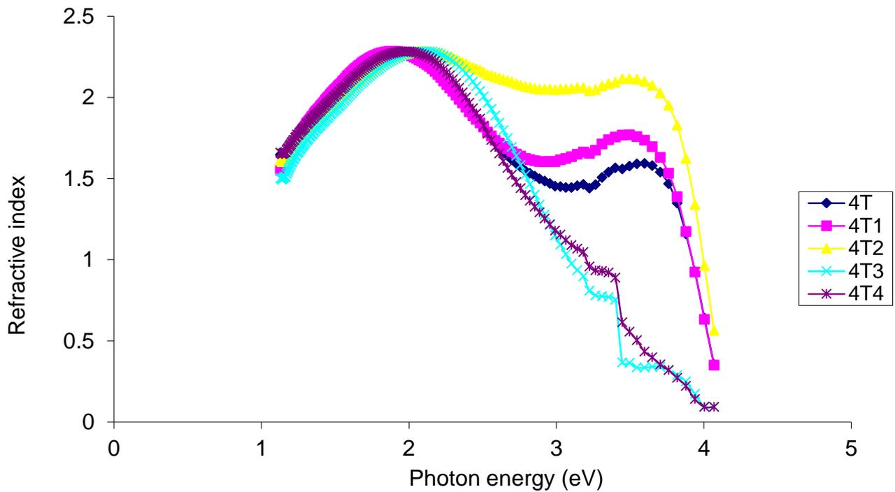
Fig. 2: Refractive index vs. photon energy for TiO<sub>2</sub>/CoO core-shell thin films
