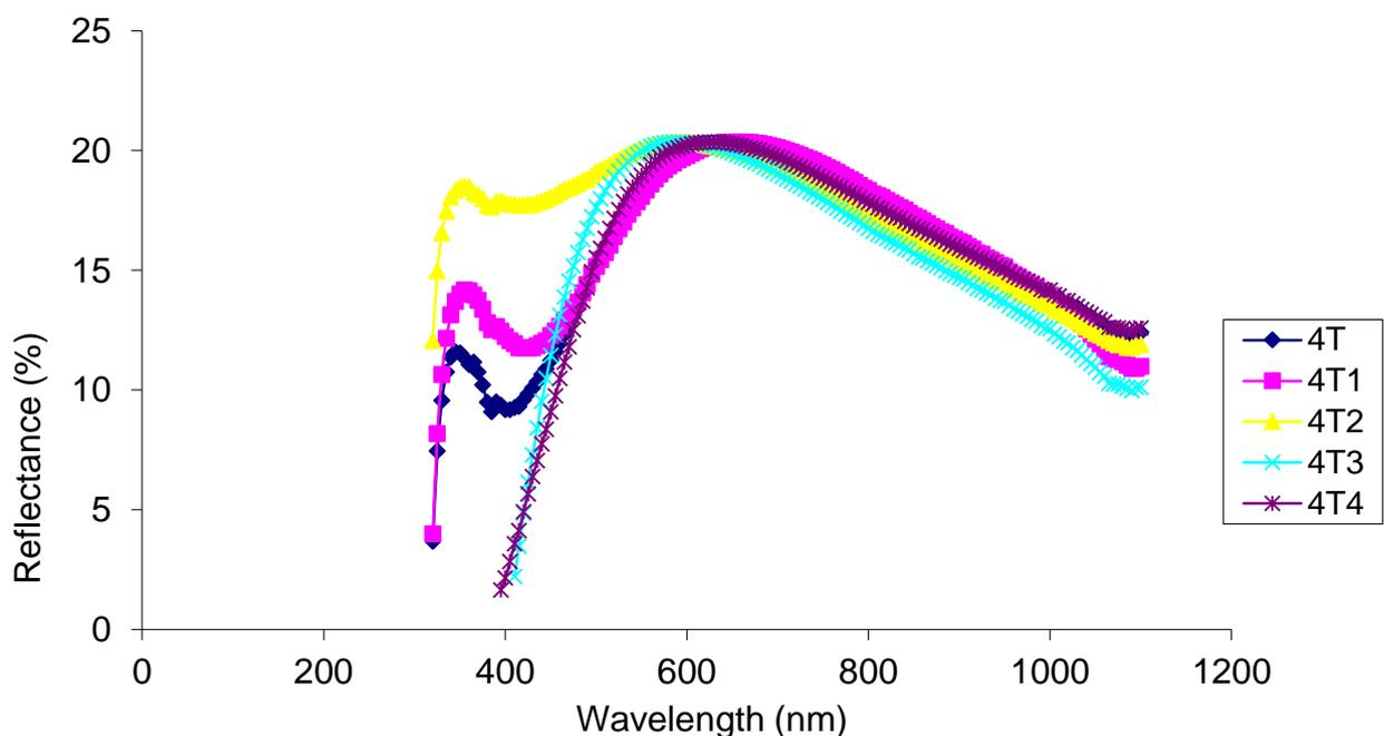
Fig. 3: Reflectance vs. wavelength for TiO<sub>2</sub>/CoO core-shell thin films
