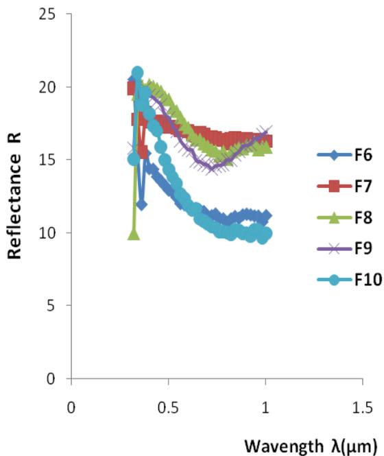
**Fig. 3: Spectral reflectance of CuNiS thin film (Slide F<sub>6</sub>-F<sub>10</sub>)**
