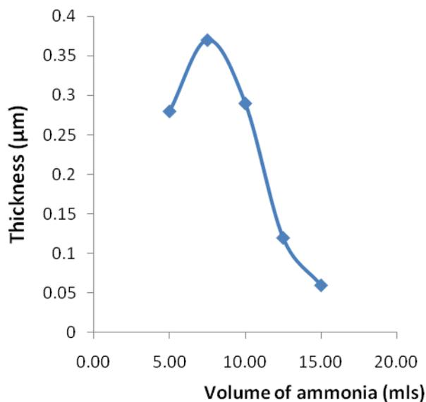
**Fig. 5: Variation of thickness with volume of ammonia for CuNiS thin film (slide F<sub>6</sub>-F<sub>10</sub>)**
