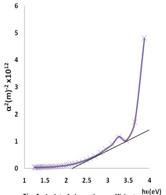
**Fig. 4 A plot of absorption coefficient squared versus photon energy for F<sub>6</sub> - F<sub>10</sub>**
