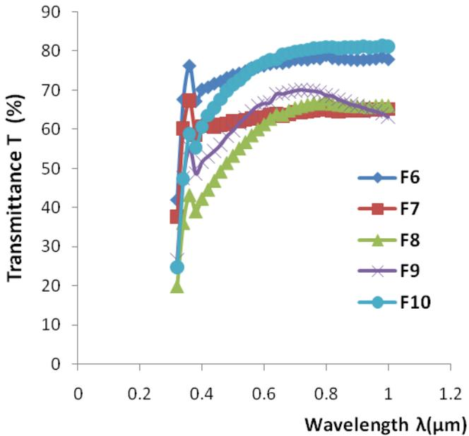
**Fig. 1: Spectral transmittance of CuNiS thin film (Slide F<sub>6</sub>-F<sub>10</sub>)**
