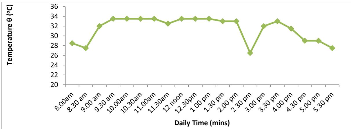
Fig. 13: Plot of Temperature (θ) against Daily Time (T) of the PV Module in Sunlight (8.00 am - 5.30 pm) for the Month of March
