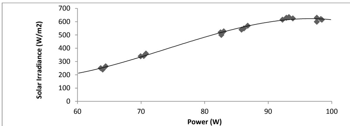
Fig. 8: Graph of Solar Irradiance (H) against Power (P) of the PV Module in Sunlight (8.00 am - 5.30 pm) for the Month of March
