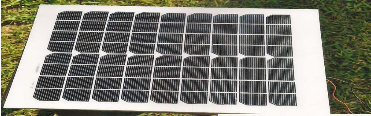
Fig. 1 Mono Crystalline Silicon Solar Panel with specifications AT-5020, 20W
