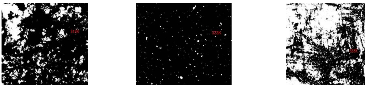
Fig.2 Micrograph images of CuAlSe 2 films grown at temperatures 313K, 333K and 353K.
